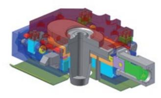
The Sliding Gate System TRS-1000L provides multiple advantages for an easier use and higher performance: Simplicity: reduction of components, quicker application on the ladle, Interchangeability with existing systems,
